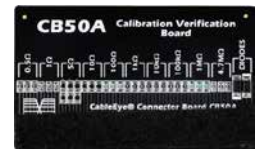
CB50A Calibration Verification Board (Item 780A)
