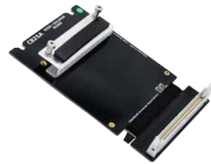
CB25A Riser Board Serves as Header Isolator Adapter for CB Boards
