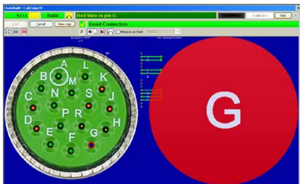
AutoBuild Screen Image Setup for 1st-Sided pinning. Target pin highlighted and read aloud.
