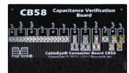
CB58 Capacitance Calibration Verification Board (Item 788)
