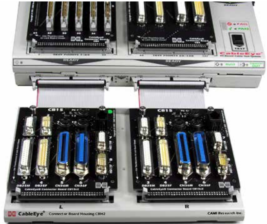
QuickMount Housing (Item 712H) CB15C connector boards (not included) shown mounted to illustrate function.
